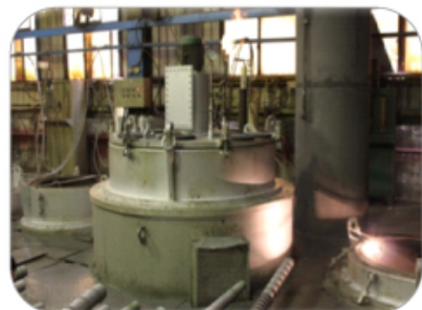
Gas Nitride Furnace
